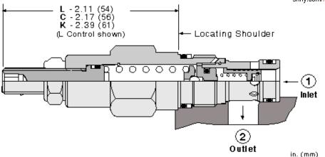
Pilot-operated, balanced-piston relief cartridges are normally closed pressure regulating valves. When the pressure at the inlet (port 1) reaches the valve setting, the valve starts to open to tank (port 2), throttling flow to regulate the pressure. These valves are accurate, have low pressure rise vs. flow, they are smooth and quiet, and are moderately fast.
